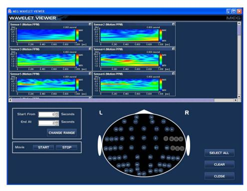
Figure 10. Visualization of the results of wavelet analysis for selected sensors. The numbers within oval shape diagram indicate the sensor number.
