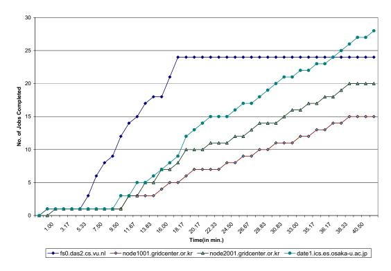
Figure 9. Scheduling with cost-time optimization: cumulative graph of the number of jobs completed versus time.
