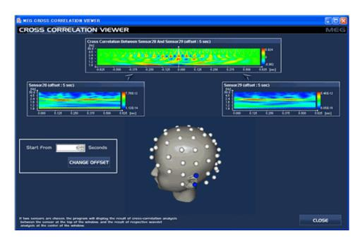
Figure 11. Visualization of the results of two different sensors data cross-correlation analysis.
