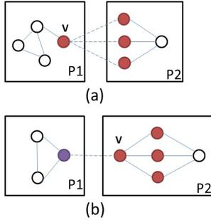
Fig 3. The role of high degree border vertices in reducing network traffic
