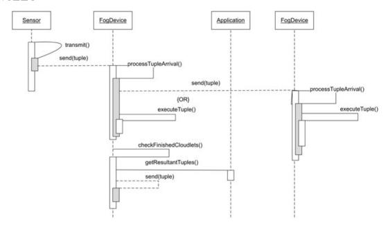
FIGURE 6 Sequence diagram of the generation and execution
