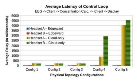
**FIGURE 11** Average delay of control loop. [Colour figure can be viewed at wileyonlinelibrary.com]
