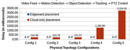
FIGURE 14 Average delay of control loop. [Colour figure can be viewed at wileyonlinelibrary.com]
