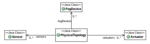
**FIGURE 5** *iFogSim* physical topology classes. [Colour figure can be viewed at wileyonlinelibrary.com]
