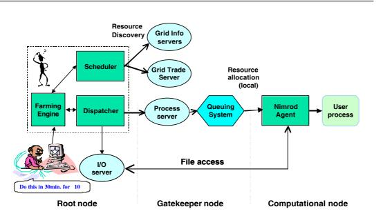
Figure 4. Nimrod-G Grid resource broker architecture.
