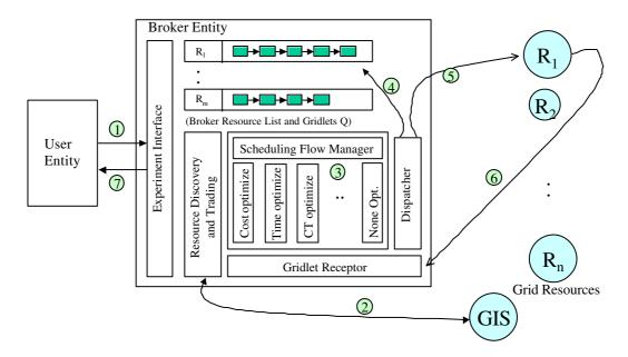
Figure 18. Economic-based Grid resource broker architecture and its interaction with other entities.
