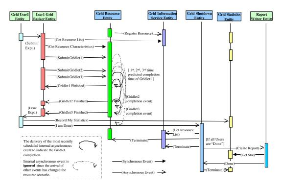
Figure 5. An event diagram for the interaction between a time-shared resource and other entities.
