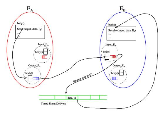
Figure 4. Entity communication model via its Input and Output entities.
