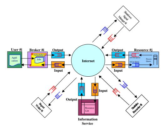
Figure 3. A flow diagram in GridSim based simulations.
