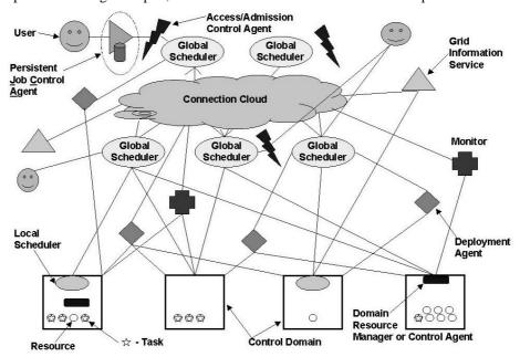
Figure 2: Hierarchical Model for Grid Resource Management.
