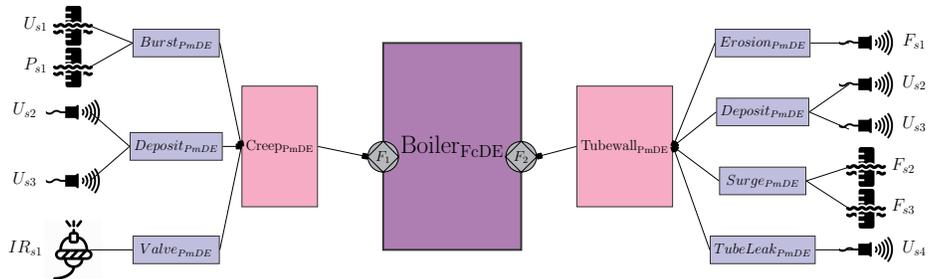
Fig. 1. Boiler Predictive Maintenance Engine
