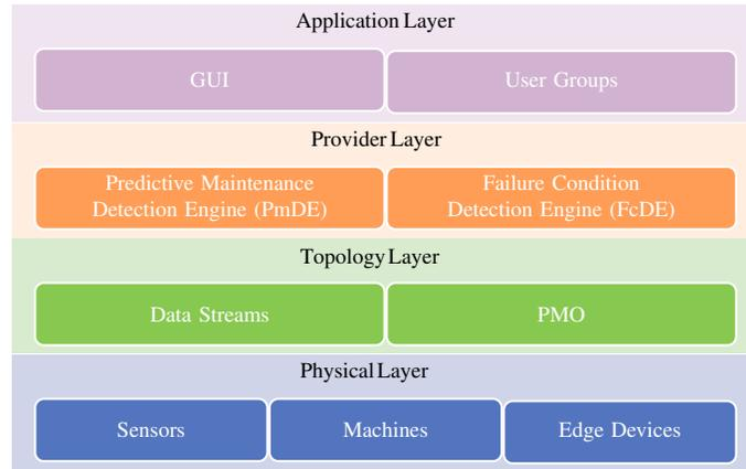
**Fig. 3.** PdM Component Architecture
