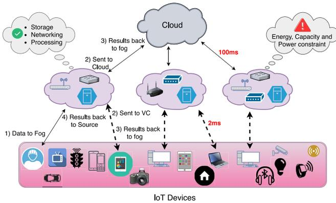
Fig. 2. Generic architecture of our proposed VSFC scheme.
