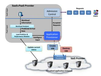
Fig. 1. Proposed mechanism for adaptive virtual machine provisioning.
