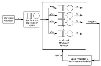
Fig. 2. Queueing model for the data center.
