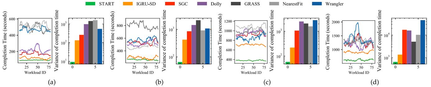
Fig. 8. Comparison of performance based on execution time for different utilization: a) utilization limit = 20%, b) utilization limit = 40%, c) utilization limit = 60% and d) utilization limit = 80%.
