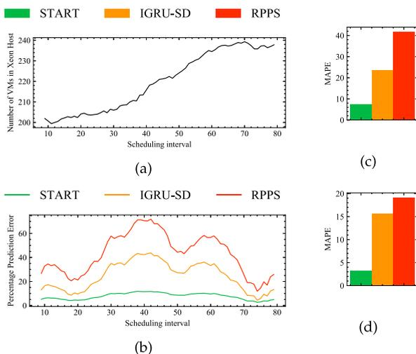
Fig. 9. Comparison of prediction accuracy of START with IGRU-SD and RPPS. (a) Number of VMs in Xeon host out of total 400 VMs, (b) Comparison of percentage prediction error, (c) MAPE values for modified environment with changing host resources (d) MAPE values for initial setup described in Section 5.
