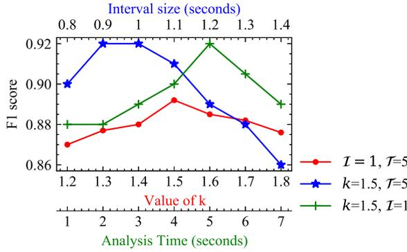
Fig. 2. Empirical results for different hyper-parameter values comparing F1 scores of straggler classification on test data.  $k$ ,  $\mathcal{I}$  and  $\mathcal{T}$  are defined in Sections 3.1 and 3.2. F1 score is defined as per Eq. (5).
