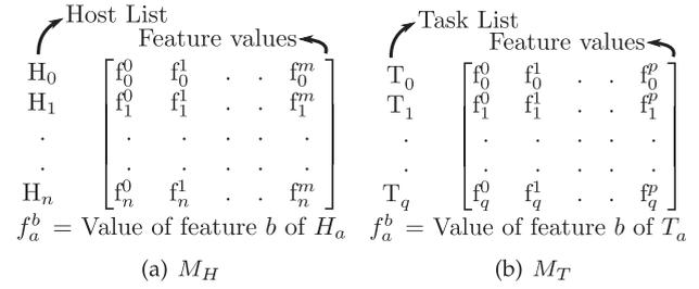
Fig. 3. Matrix representation of model inputs.
