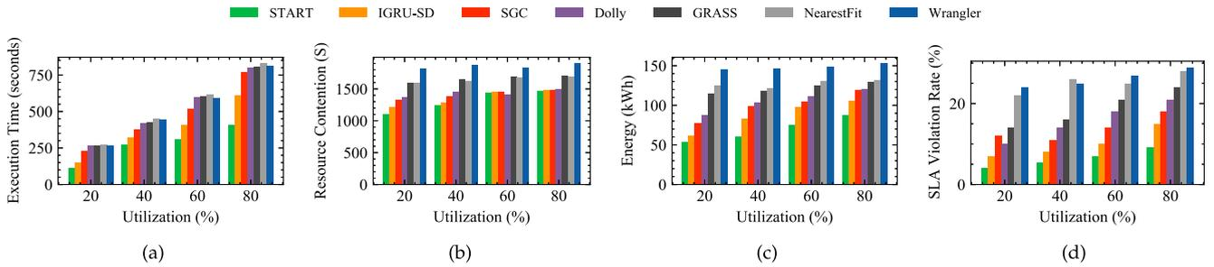
Fig. 6. Comparison of QoS parameters with different value of CPU, disk, network and memory Utilization: a) Execution Time, b) Resource Contention, c) Energy Consumption and d) SLA Violation Rate
