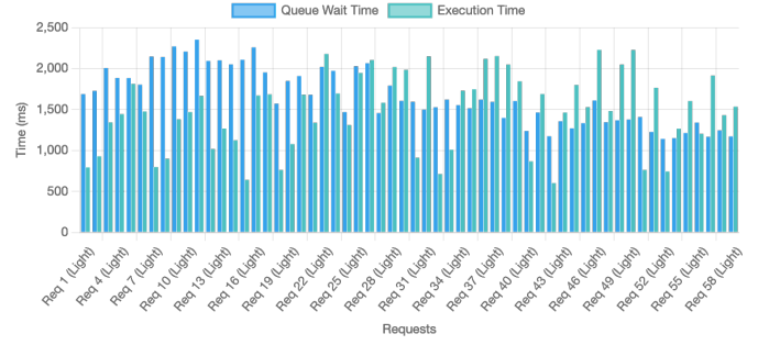
Fig. 4. Impact of Request Queue and Cold Start on Function Request Performance
