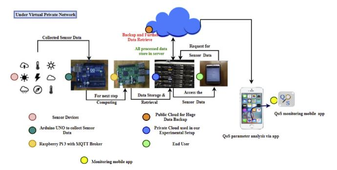
Fig. 9. Experiment setup for collecting sensor data, upload and monitoring via QoS monitoring application.
