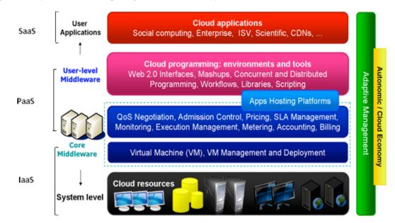
Figure 6. Layered Cloud computing architecture. (Buyya et. al 2009)
