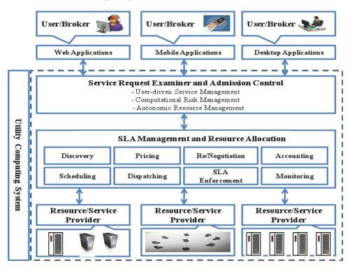
*Figure 2. SLA-oriented utility computing system architecture*
