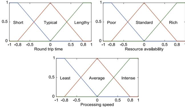
Fig. 7. Membership function of status metrics parameters.
