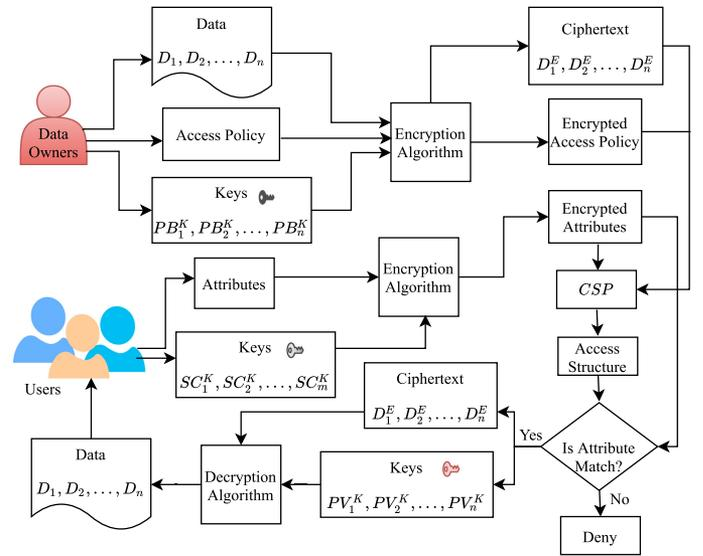
Fig. 2. Data encryption and decryption in MLPAM.
