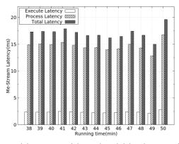
**Fig. 6.** Statistics of execute delay, process delay and total delay data sets of the Me-Stream optimization strategy on the WordCount instance.
