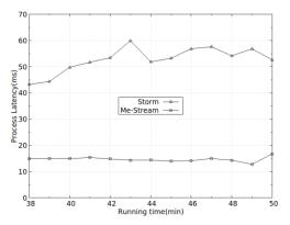
**Fig. 4.** Comparison of process latency between the default scheduler and Me-Stream on the WordCount instance.
