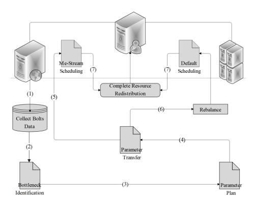
Fig. 1. Elastic scaling process of operator parallelism strategy (Me-Stream).
