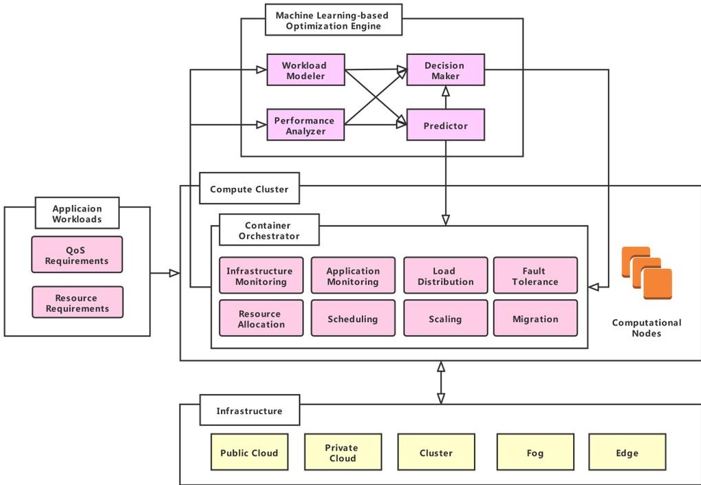
Fig. 2. A high-level machine learning-based container orchestration framework reference architecture.
