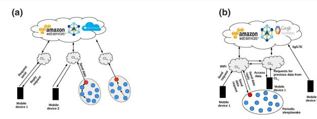
FIGURE 7 (a) Architecture of MCC-WSN integration. (b) Mobility Scenarios of mobile user
