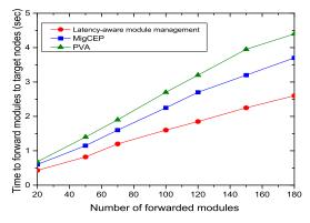
Fig. 8. Required time for Application Module forwarding vs number of forwarded modules.
