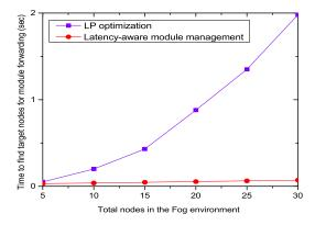
Fig. 7. Required time for generating LP and heuristic solution.
