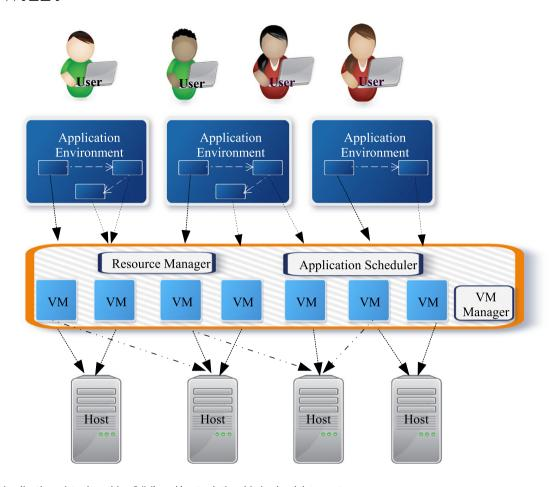
FIGURE 1 Application, virtual machine (VM), and host relationship in cloud data center
