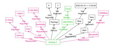
Fig. 15. Sub-intent obtained after Non-Functional Decomposition of intent to host feature C on Cloud.
