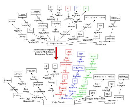
Fig. 11. Functional Decomposition of an intent identifying required VNFs/PNFs and deployment domains.
