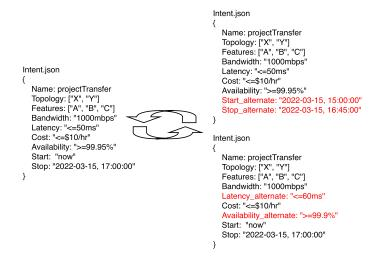
Fig. 10. Intent negotiation generating alternate solutions with relaxed temporal and resource requirements during system's inability to satisfy an intent because of resource scarcity.
