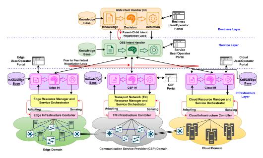
Fig. 3. Multi-layered IDSM system architecture consisting layered arrangement of intent handlers, control loops and autonomous domains of edge, CSP and cloud.
