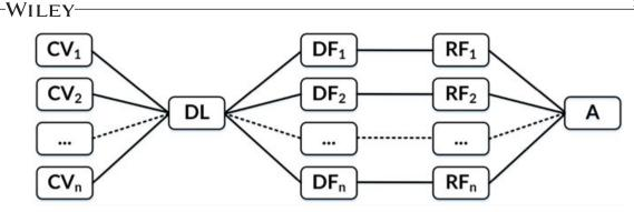
**FIGURE 7** The intelligent surveillance systems face recognition workflow implemented using Apache NiFi [Colour figure can be viewed at wileyonlinelibrary.com]
