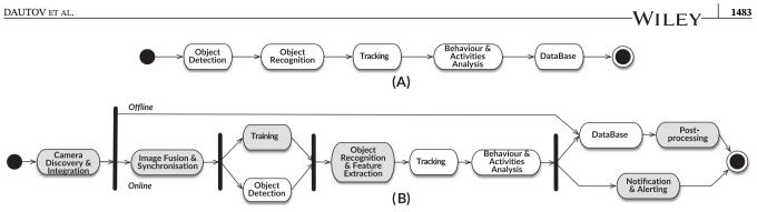
FIGURE 4 (A) Intelligent surveillance systems and (B) metropolitan intelligent surveillance system reference workflows
