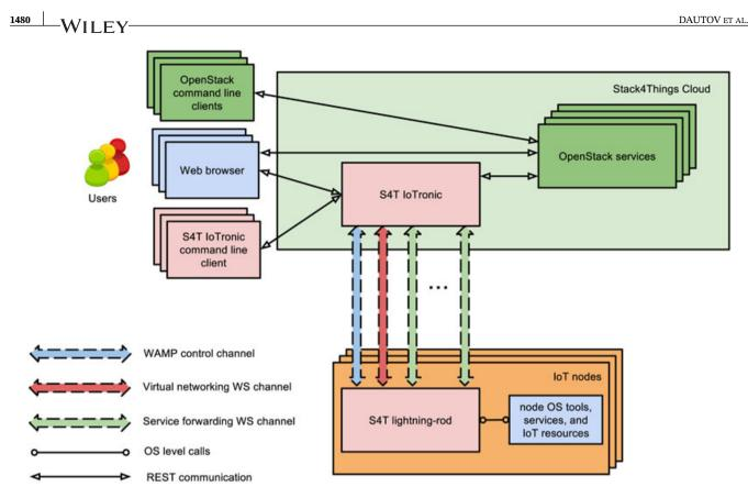
**FIGURE 2** A bird's eye view on the Stack4Things (S4T) architecture. IoT, Internet of Things; REST, Representational State Transfer; WAMP, Web Application Messaging Protocol; WS, WebSocket [Colour figure can be viewed at wileyonlinelibrary.com]
