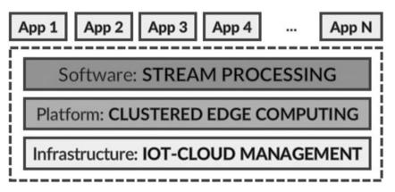
FIGURE 1 Conceptual architecture of the metropolitan intelligent surveillance system framework. IoT, Internet of Things
