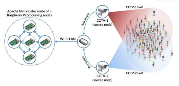
**FIGURE 8** A metropolitan intelligent surveillance system scenario implemented by clustered edge computing. LAN, local area network [Colour figure can be viewed at wileyonlinelibrary.com]
