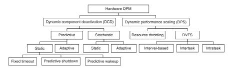
FIG. 6. DPM techniques applied at the hardware and firmware levels.
