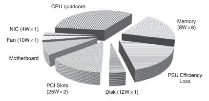
FIG. 2. Power consumption by server's components [5].
