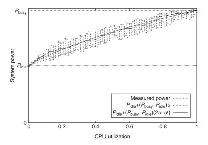
FIG. 3. Power consumption to CPU utilization relationship [10].
