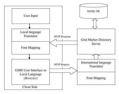
Figure 2: Architecture for localization of GMD user interface.
