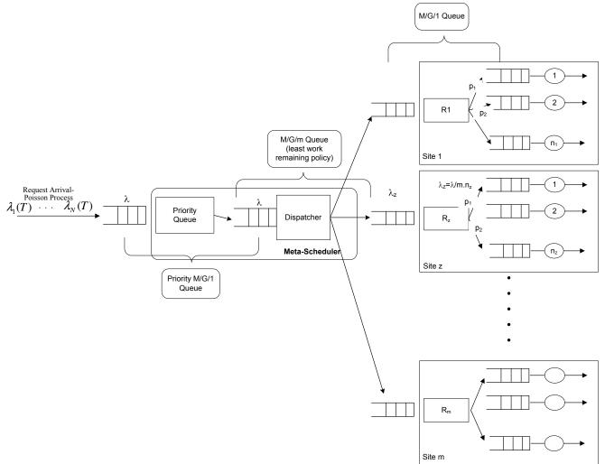
FIGURE A.1. Queuing Network Model of Meta-scheduling
