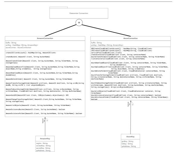
Fig. 4: Datacenter Conection package for connecting to AWS and Azure datacenters
