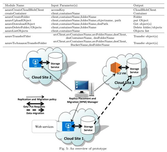
and migration (RPM) manager. The RPM manager makes decision on replica placement and migration across data stores based on the proposed heuristic solution [14]. The RPM issues Http requests (REST call) to the VMs deployed in cloud sites and receives Http responses (JSON objects). The VMs process the received requests via the deployed web services that are
