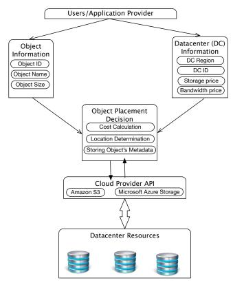
Fig. 2: Key architectural components of object placemnt across cloud-based data stores
