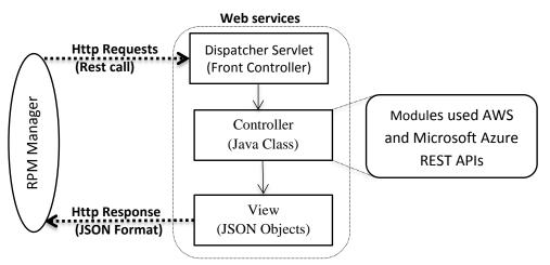
Fig. 6: Web services components used in the prototype
