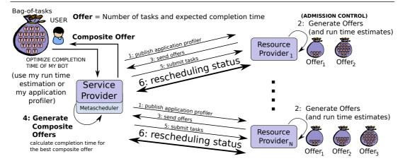
Figure 1. Components' interaction to schedule a Bag-of-Tasks on multiple resource providers.
