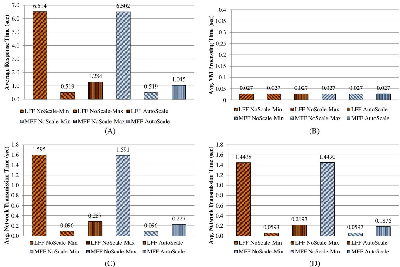
**FIGURE 6** Average response and processing time with various autoscaling policies. A, Average response time; B, Average processing time at three-tier application servers; C, Average network delays enforcing through service function chaining (SFC) policies; D, Average network delays through SFC policies without intrusion detection system (IDS). LFF, least full first; MFF, most full first [Colour figure can be viewed at [wileyonlinelibrary.com](http://wileyonlinelibrary.com)]
