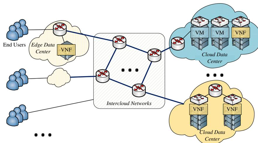
**FIGURE 1** Architecture of network functions virtualization (NFV) in edge-cloud environments. VM, virtual machine; VNF, virtualized network function [Colour figure can be viewed at [wileyonlinelibrary.com](http://wileyonlinelibrary.com)]
