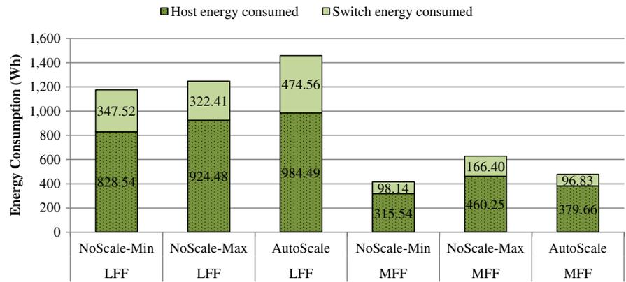
**FIGURE 9** Energy consumption in hosts and switches in the data center. LFF, least full first; MFF, most full first [Colour figure can be viewed at [wileyonlinelibrary.com](http://wileyonlinelibrary.com)]
