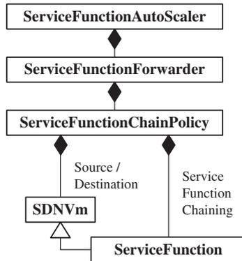
**FIGURE 3** Class diagram for simulating service function chaining
