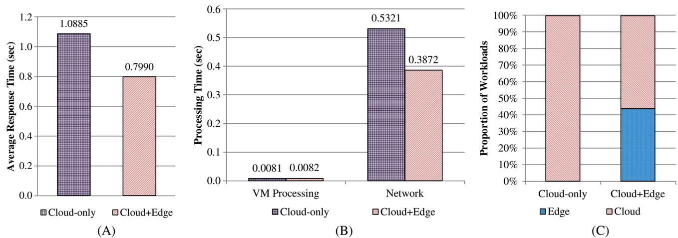
**FIGURE 10** Performance evaluation results of virtualized network function (VNF) placement policies in edge-cloud environment. A, Average response time; B, Virtual machine (VM) processing time at application servers and network transmission time including service function chaining (SFC) delays; C, Workload proportion [Colour figure can be viewed at [wileyonlinelibrary.com](http://wileyonlinelibrary.com)]
