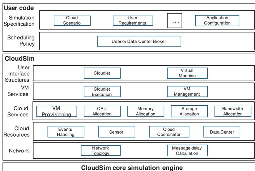
Figure 3. Layered CloudSim architecture.
