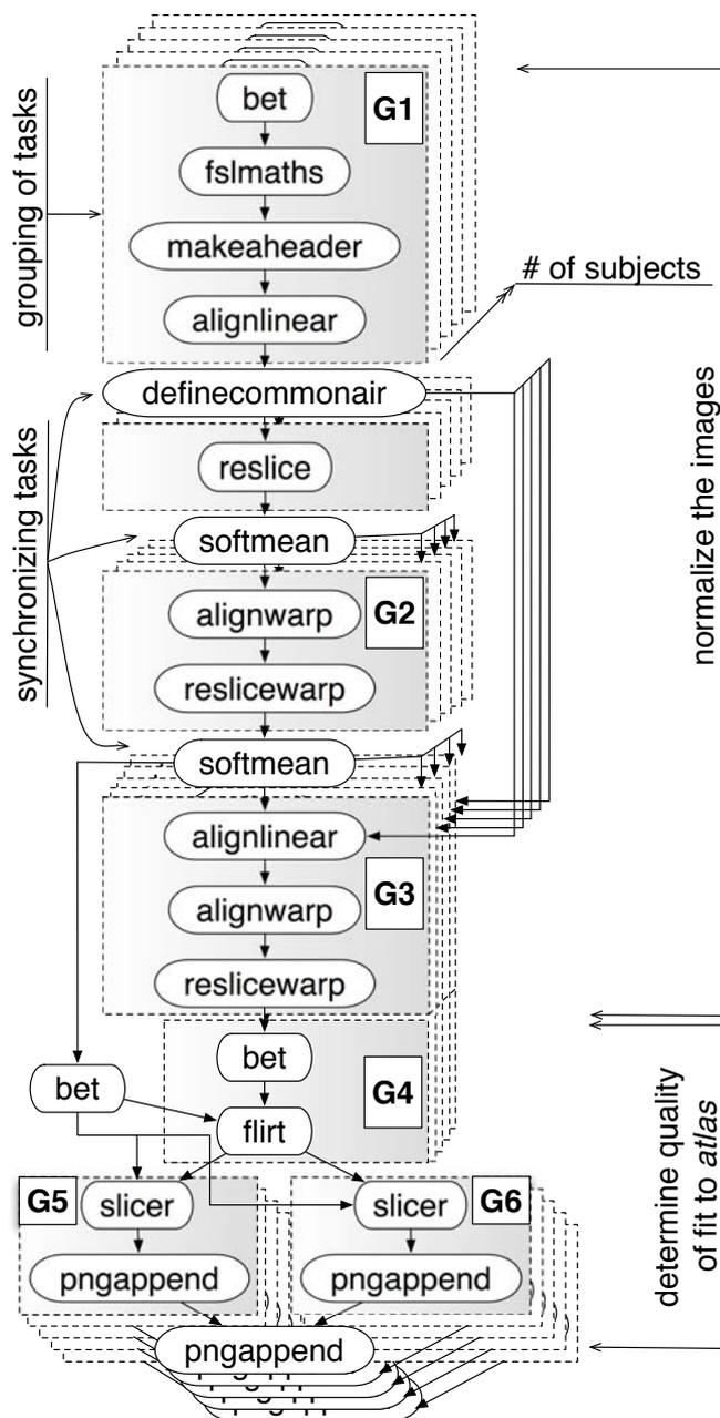
FIGURE A.1: Image Registration application as a workflow.
