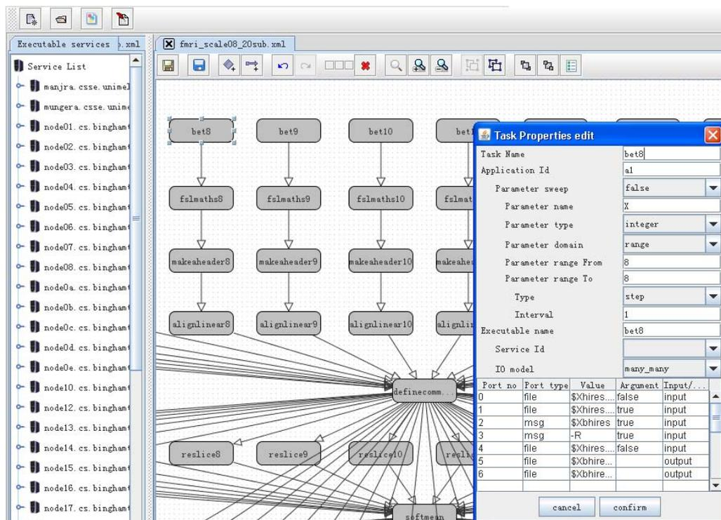
FIGURE 3.4: The workflow editor showing the Image Registration application workflow and its parameters.
