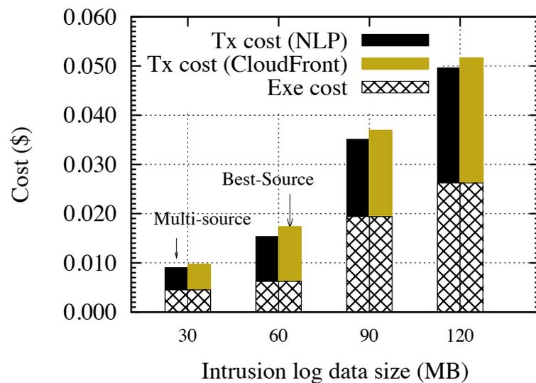
FIGURE 4.7: Comparison of total cost when both computation and transfer costs are non-zero.
