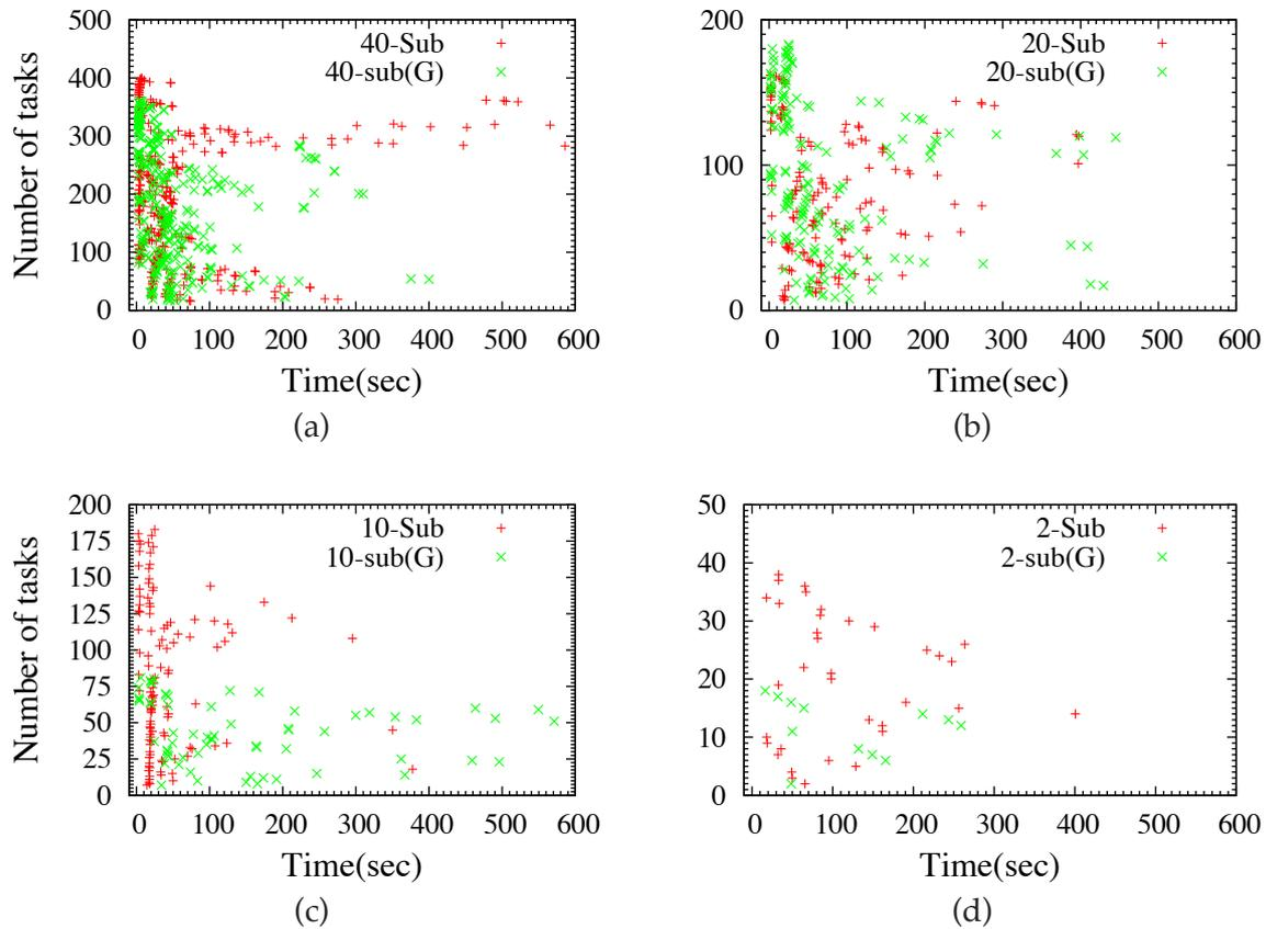
**FIGURE 3.15:** Number of tasks executed in time: Parallelism that was achieved in the system. (a) Number of tasks executed in time for 40 subjects. (b) Number of tasks executed in time for 20 subjects. (c) Number of tasks executed in time for 10 subjects. (d) Number of tasks executed in time for 2 subjects.
