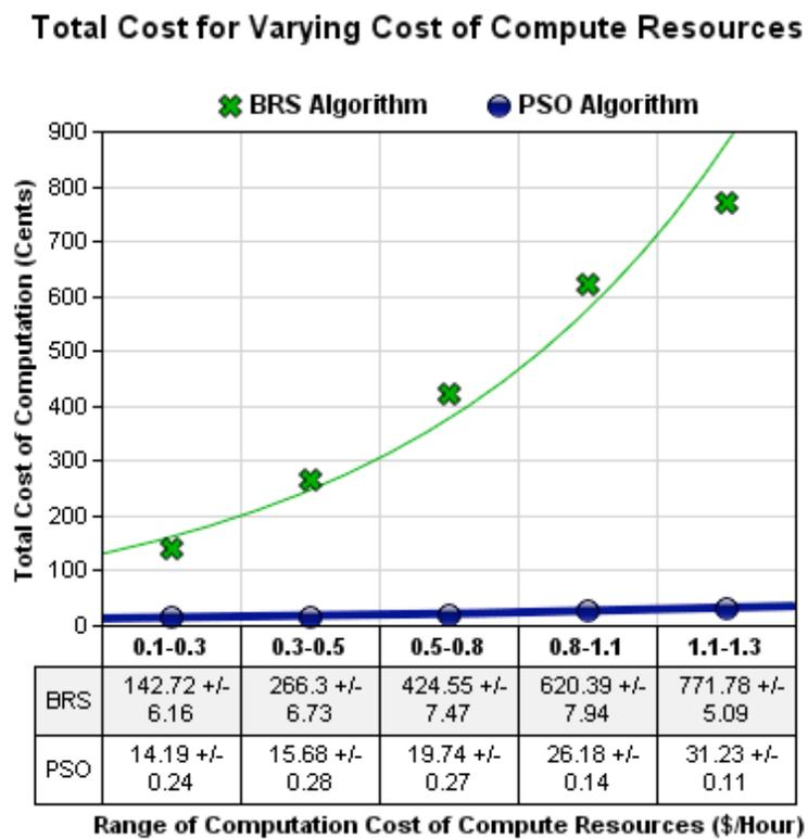
**FIGURE 6.5:** Comparison of total cost between PSO based resource selection and best resource selection algorithms when varying computation cost of all the resources ( for 128MB of data).
