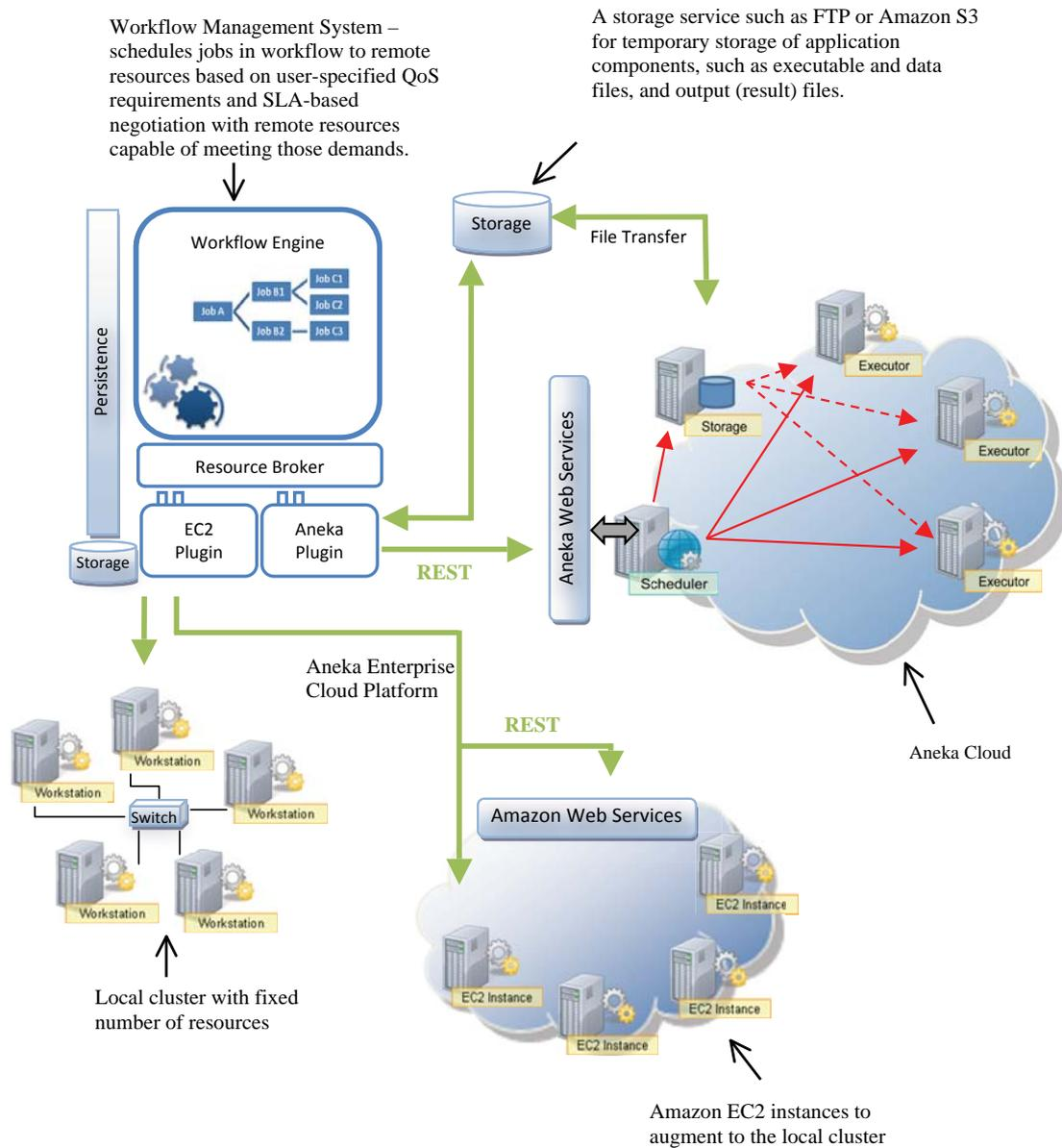
FIGURE 3.10: Integration of workflow engine with Grids and Cloud
