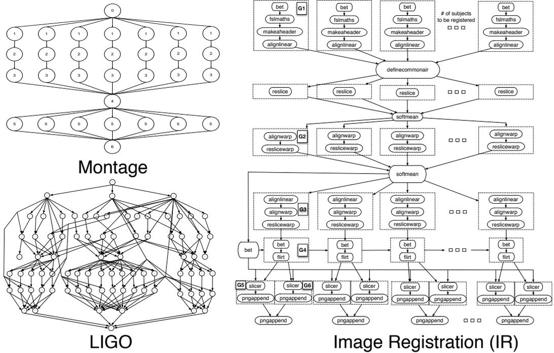
**FIGURE 5.4:** Application Workflow types: Balanced (Montage), complex (LIGO) and hybrid (IR) workflows
