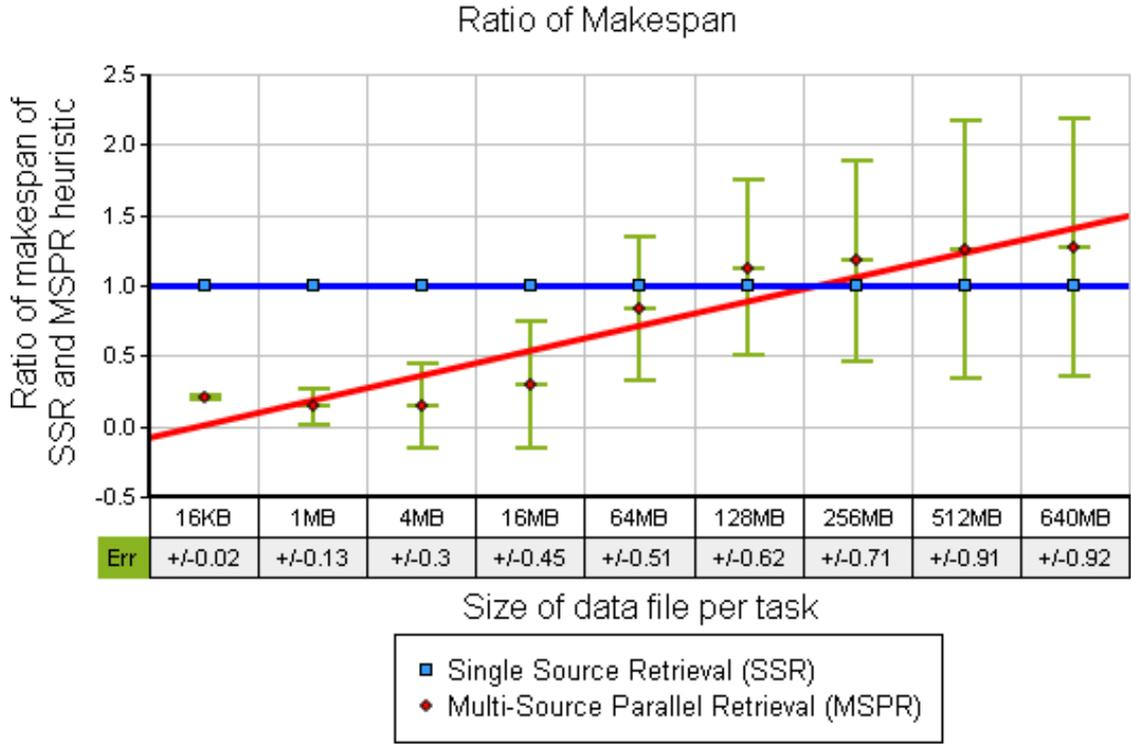
**FIGURE 5.11:** Determining the benefit of using multi-source parallel data retrieval by comparing the ratio of makespan for IR workflow (WF type three) in real environment
