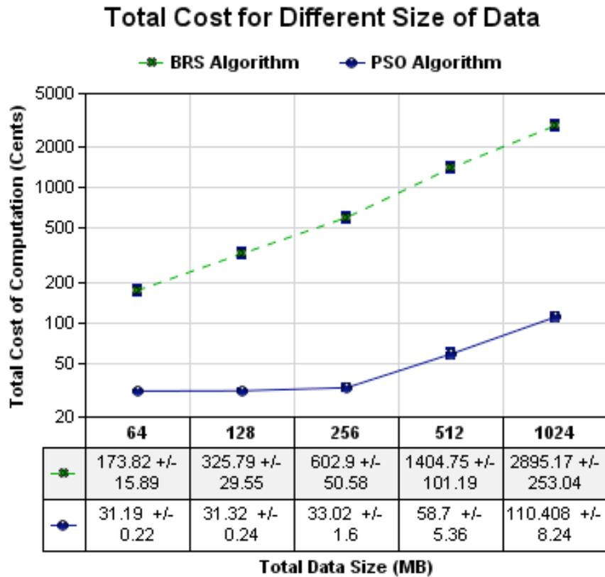
**FIGURE 6.3:** Comparison of total cost between PSO based resource selection and best resource selection algorithms when varying total data size of a workflow.
