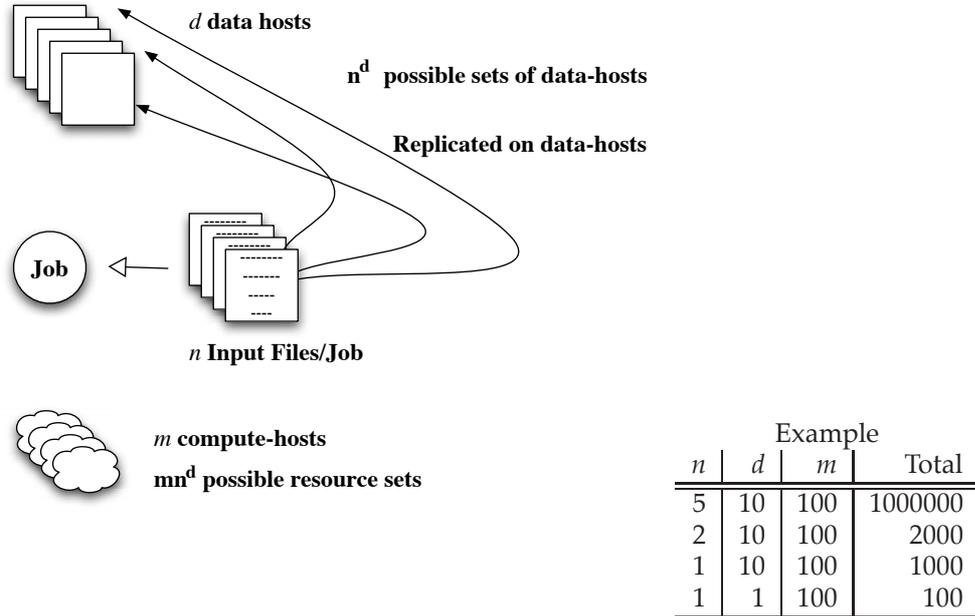
FIGURE 1.4: Datahost and Compute host selection problem for a single task.
