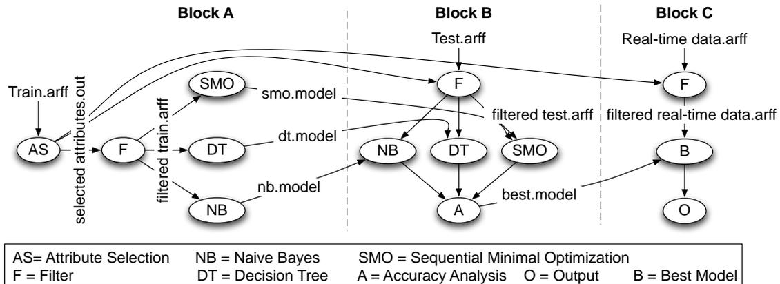
FIGURE 4.3: Intrusion Detection workflow
