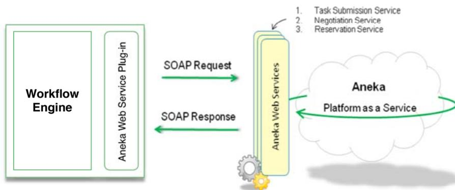
**FIGURE 3.8:** The workflow engine interacting with Aneka web services using SOAP request/response.
