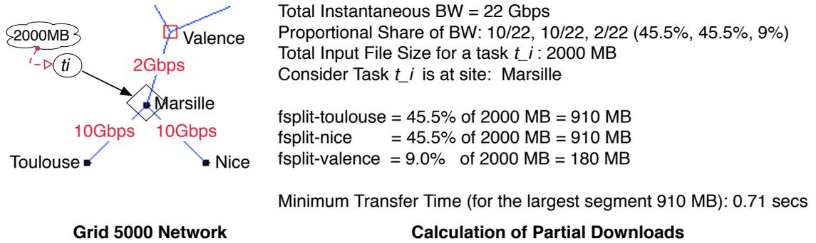
**FIGURE 5.3:** An example showing the partitioning of input files in proportion to the available instantaneous bandwidth.
