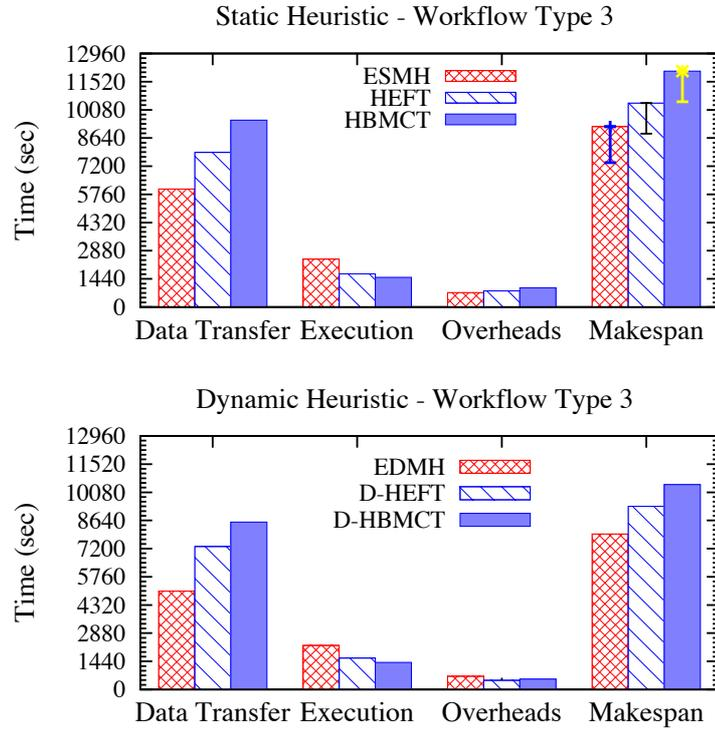
FIGURE 5.10: Makespan of IR workflow (WF 3) using static and dynamic heuristic.
