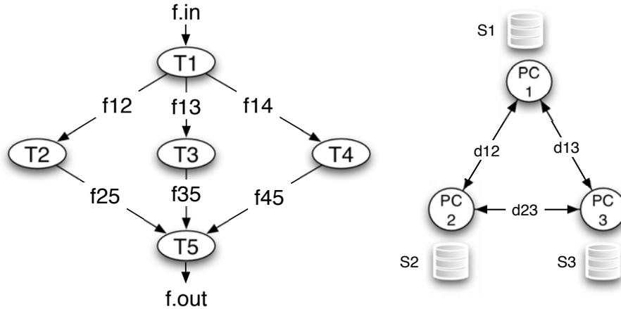
FIGURE 6.1: An example workflow, compute nodes (PC) & storage (S).
