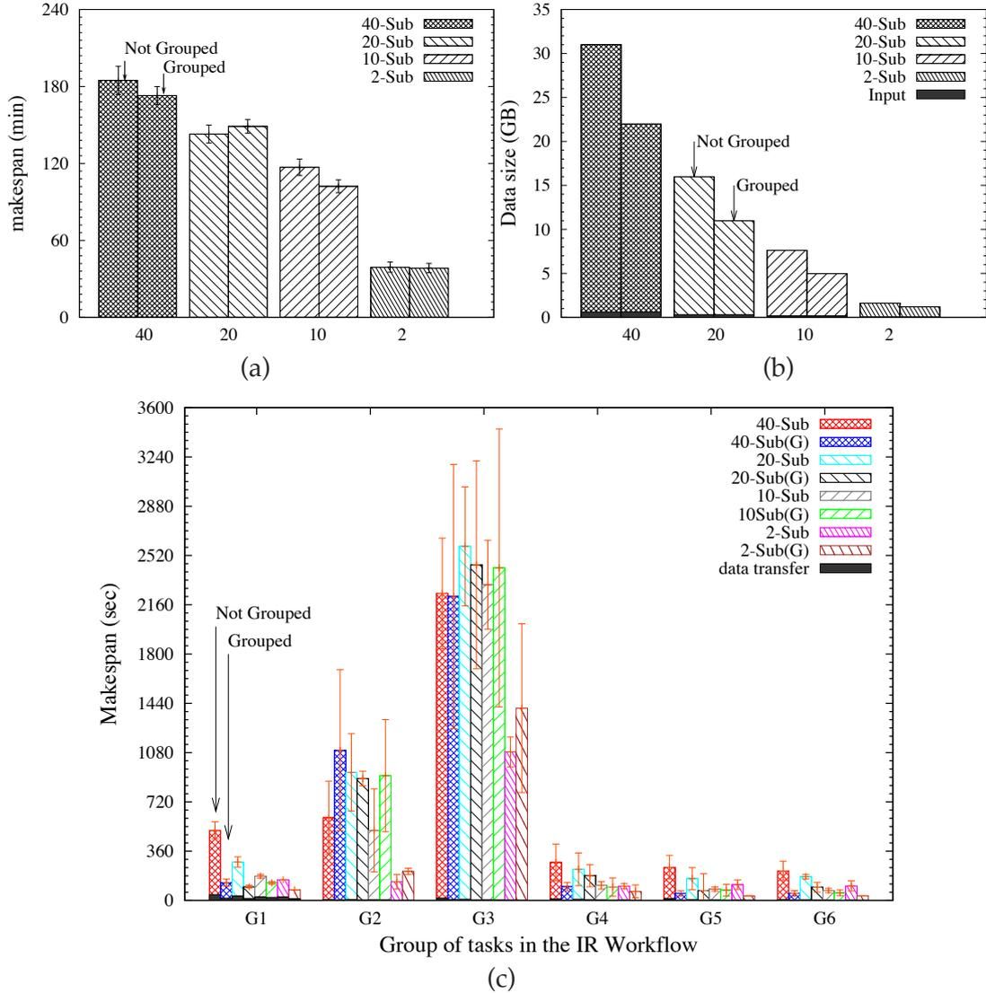
**FIGURE 3.14:** (a) Comparison of makespan of workflow according to the number of subjects used. (b) Data size according to the number of subjects used. (c) Comparison of makespan between grouped and ungrouped tasks (see Figure 3.13 for grouping of tasks).
