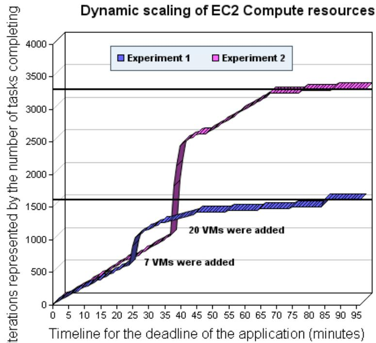
**FIGURE 3.19:** Number of tasks completing in time as the number of compute resources provisioned were increased at run-time
