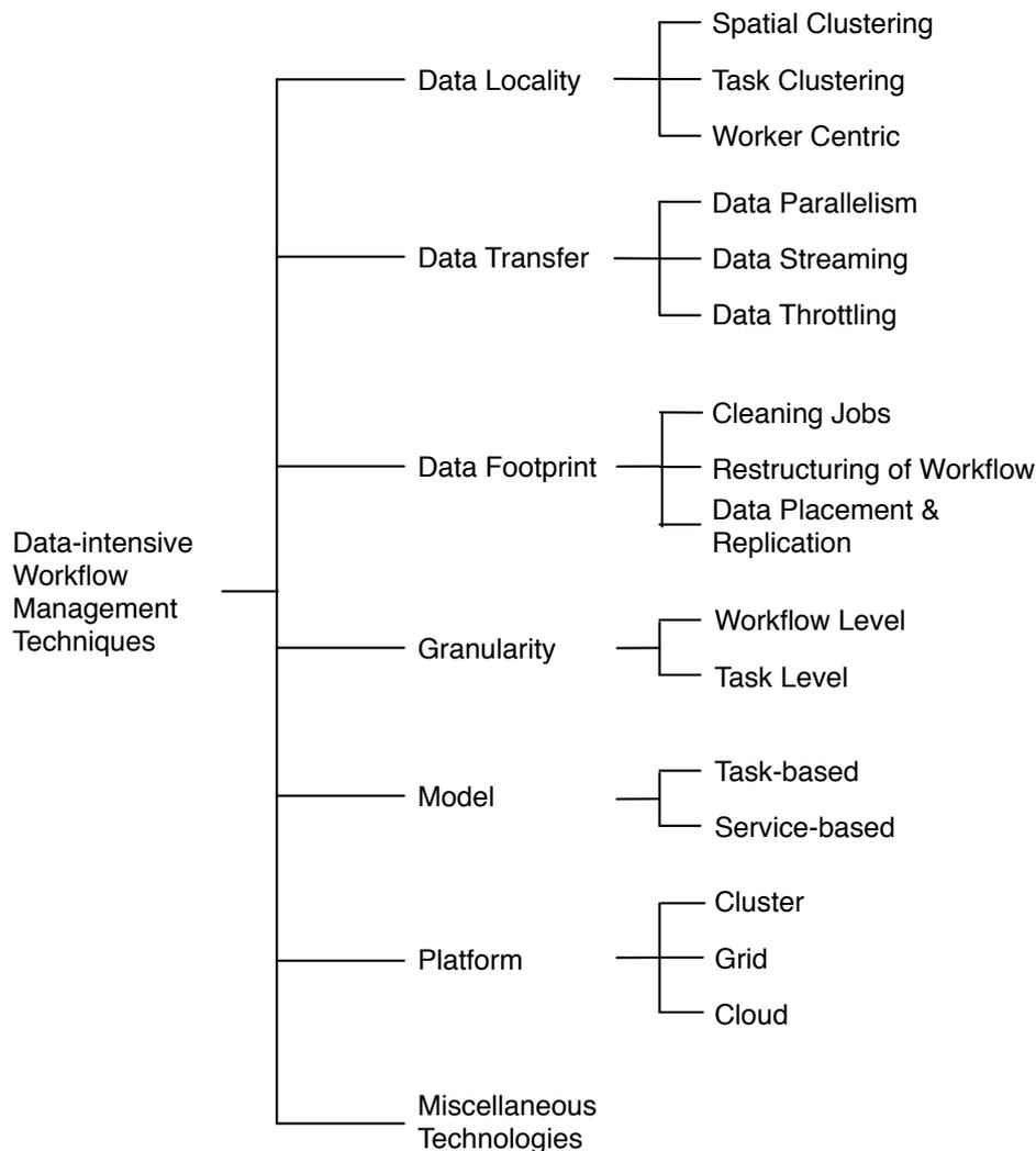
**FIGURE 2.2:** Classification of management techniques for data intensive application workflows.
