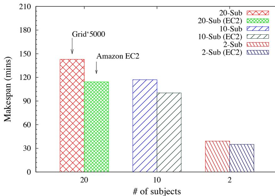
FIGURE 3.17: Makespan comparison between EC2 and Grid'5000 setups.
