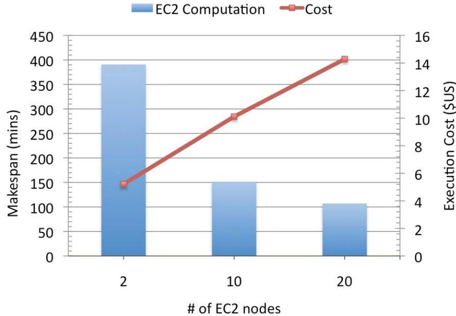
**FIGURE 3.18:** Comparison of execution time and cost when using Cloud resources.
