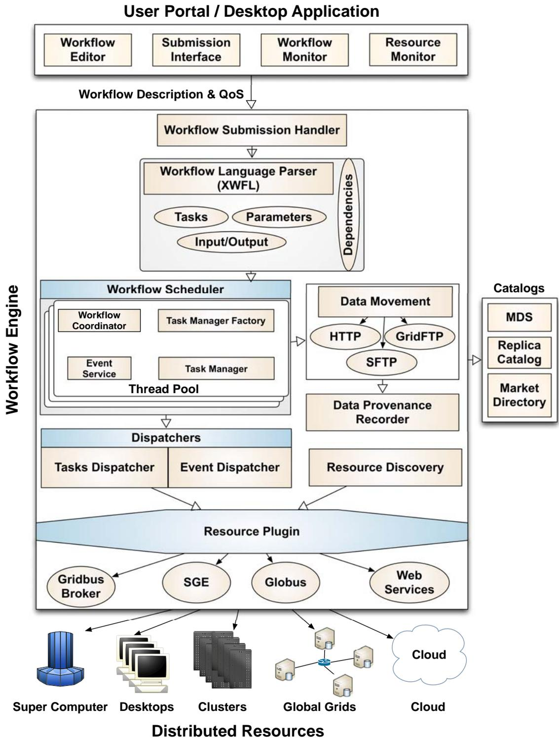
FIGURE 3.1: Workflow Management System Design.
