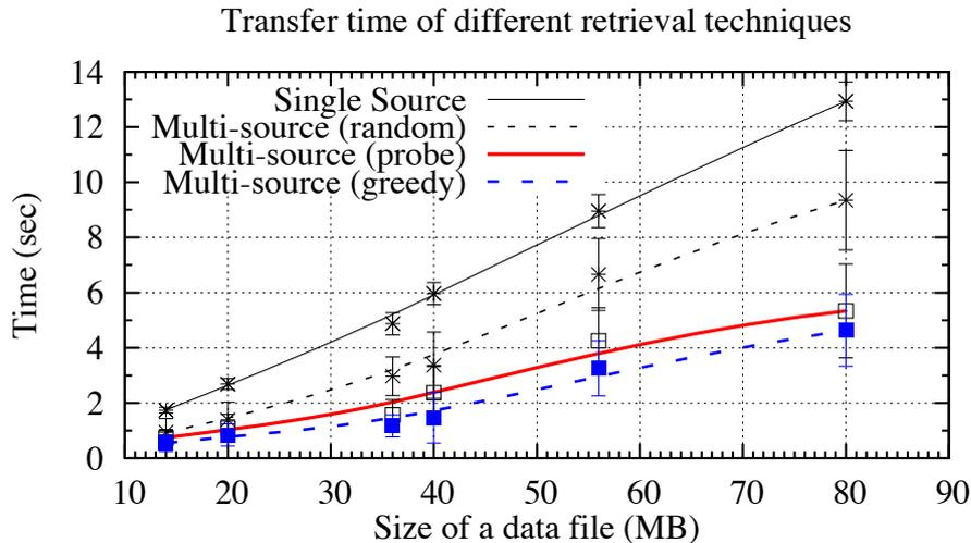
**FIGURE 5.7:** Comparison of transfer time and error margins between single-source and multi-source data retrieval techniques using data files of different sizes (files are from IR Workflow experiment only) (Bézier curve fitting used)
