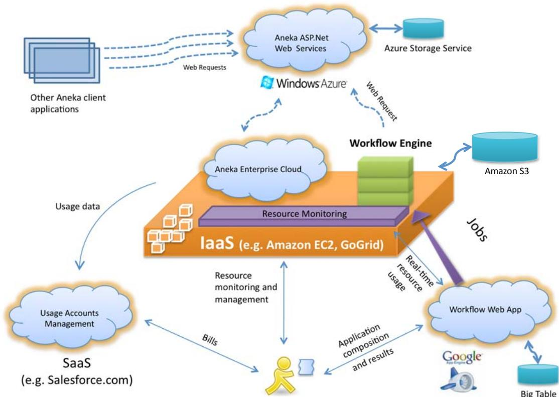
FIGURE 3.11: The workflow system utilizing various Cloud services.
