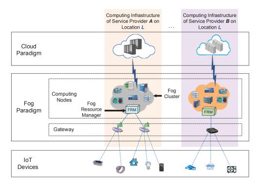
Figure 3.1: Fog environments for Edge affinity-based application management
