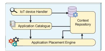
Figure 5.2: Software architecture of Fog Gateways
