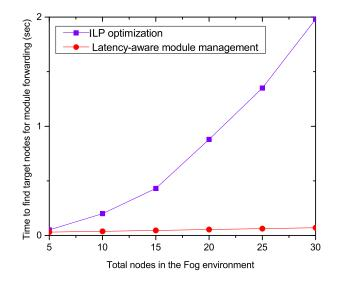
Figure 4.7: Required time for generating ILP and heuristic solutions
