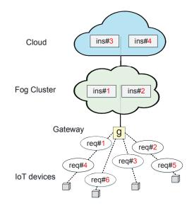
Figure 7.2: Illustrative integrated Fog-Cloud environments
