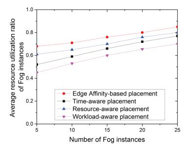
Figure 3.13: Average resource utilization for varying number of Fog instances
