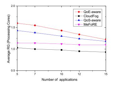
Figure 6.11: Resource gain for varying number of applications
