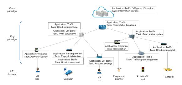
Figure 1.2: An illustration of application execution in Fog environments
