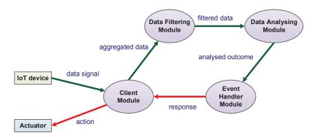
Figure 4.1: Dataflow model for a distributed application
