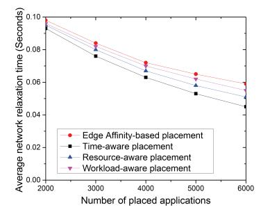
Figure 3.9: Average network relaxation for varying number of placed applications
