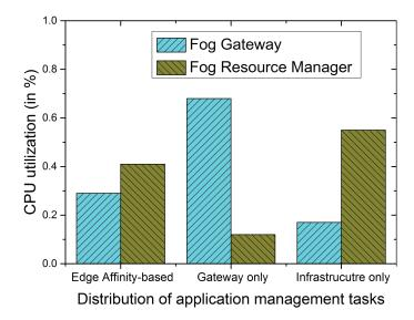
Figure 3.7: Average management load in different management setup
