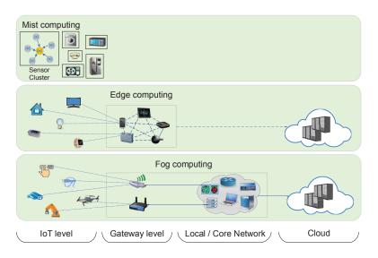
Figure 2.3: Domain of Mist, Edge and Fog computing
