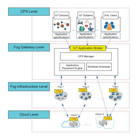
Figure 2.7: A perspective model for application management in Fog
