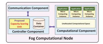
Figure 6.2: Architecture of a Fog computational node
