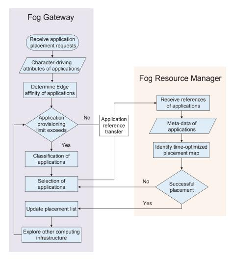
Figure 3.3: Flowchart for proposed Edge affinity-based application management
