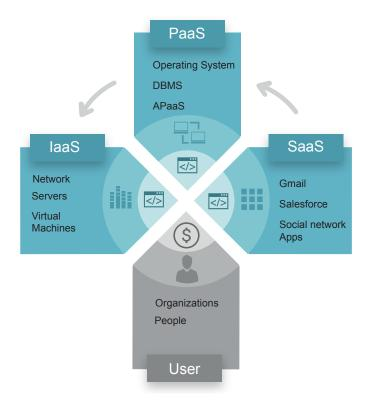
Figure 2.1: Services provided in Cloud Computing. Customers rent those computing resources and manage those resources by themselves using applications provided
