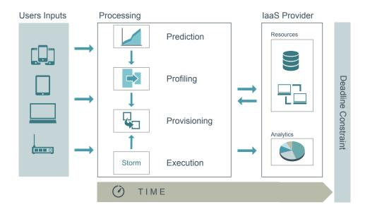
Figure 3.1: Big Data Processing Architecture. Data streams are required to be processed in cloud environment. Before that an estimation and assignment of resources are done in order to reach uses satisfaction
