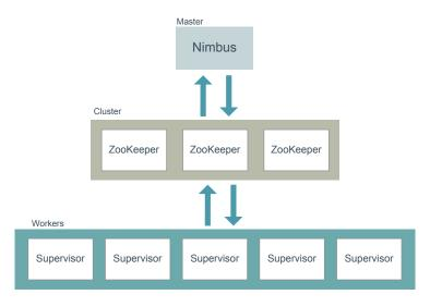
Figure 2.5: Storm Components. Master Node (Nimbus) send request of execution of task to Worker nodes (Supervisor) through Zookeeper cluster
