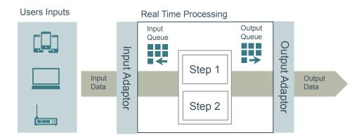
Figure 2.4: Stream Processing. Information is processed before it is saved on database
