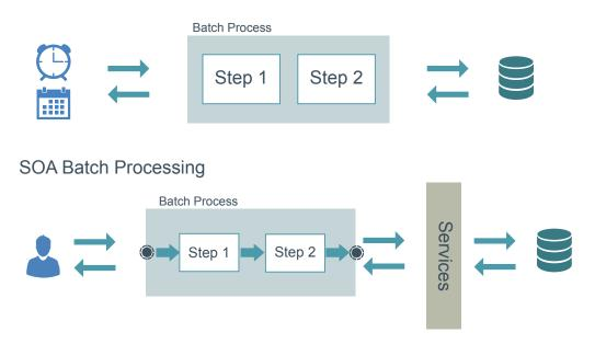
Figure 2.3: Batch Processing. Two kinds: Traditional (scheduled task) and SOA (Perform task under request)
