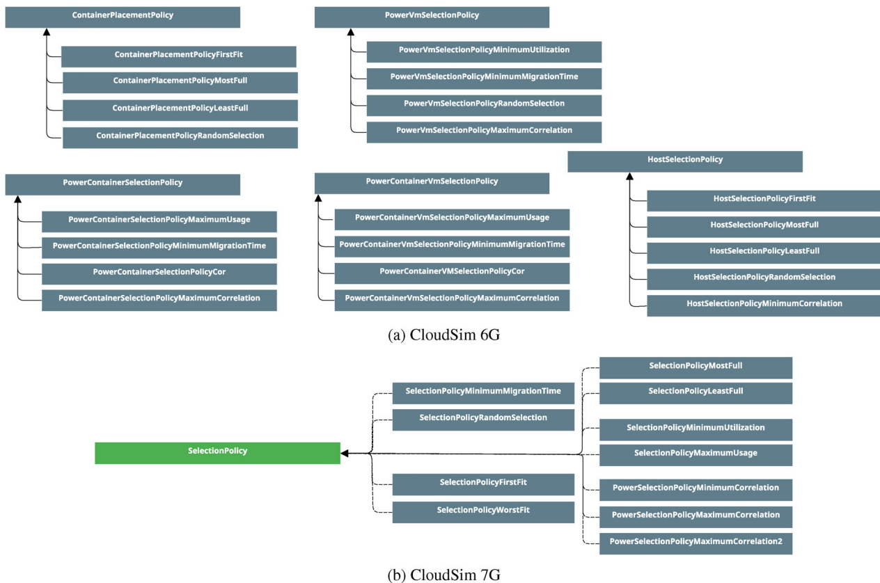
FIGURE 4 | UML class diagram of the host and guest selection policies in CloudSim. Green boxes depict Java interfaces, and blue boxes represent Java classes. The relationship arrows follow the UML relations notation style: A dashed line represents a realization/implementation, and a full line represents inheritance. Line colors are for presentation purposes only.
